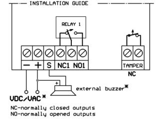
IMPORTANT! Output S must not be directly connected to (+) pole of power supply (see schema).
